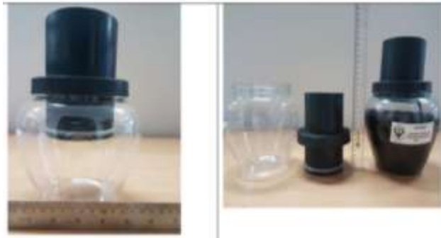
Gambar 2. Larvitrap top berbahan plastik (sumber: Roebanji et al. , 2017)
